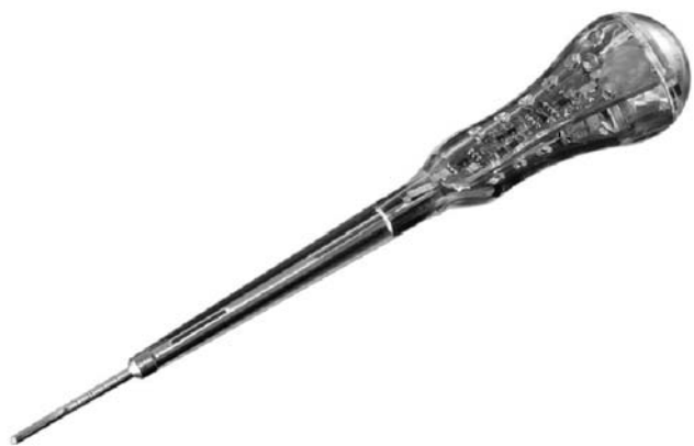
FIGURE 1. The PediGuard—electronic conductivity device.
